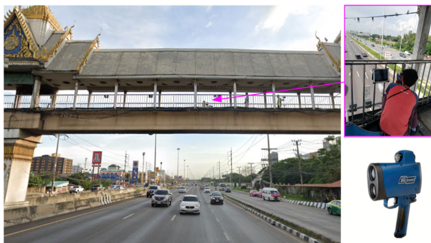
FIGURE 2. Traffic video recording and vehicle speed measurement on the skycrossing bridge over Phahonyothin road at the height 7.3m over the road. (Image on the road from Google street view)
