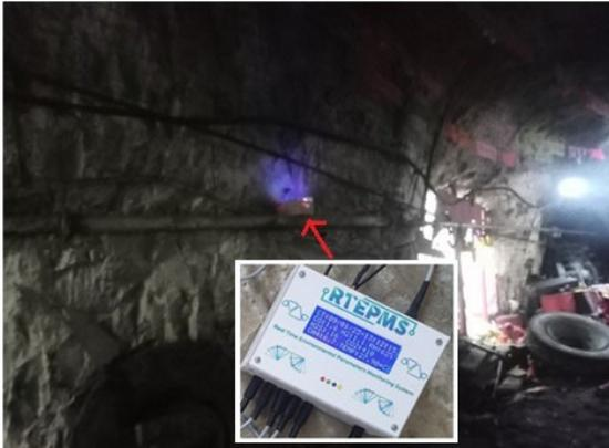
FIGURE 20. RTEPMS with LoRa transmitter deployment at level 26 of the underground mine.
