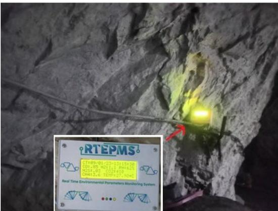
FIGURE 21. RTEPMS with LoRa receiver deployment at level 26 of the underground mine.
