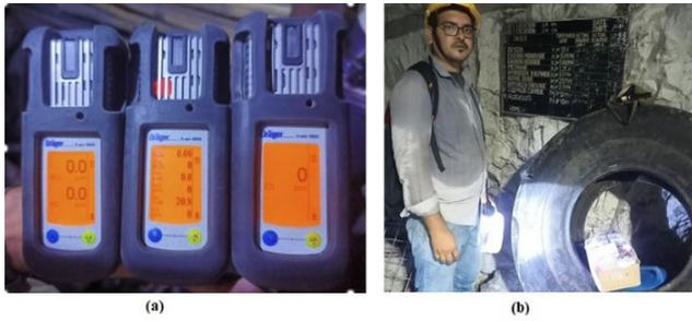
FIGURE 17. (a) Multi-gas detector device, (b) Board to display gas parameter.
