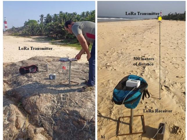
**FIGURE 16.** Establishment of wireless communication between RTEPMS transmitter and receiver.
