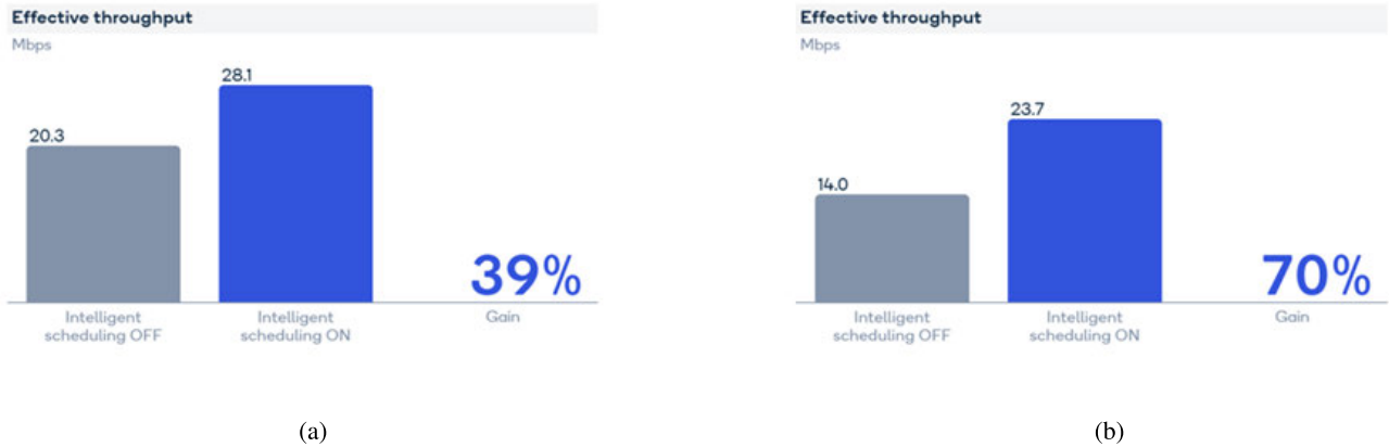
FIGURE 15. (a) Scenario A: Average effective DL throughput comparison between IAIS OFF (baseline CSI-RS based DL LA) and IAIS ON for the 5G UE in the OTA deployment, (b) Scenario B: Average effective DL throughput comparison between IAIS OFF (baseline CSI-RS based DL LA) and IAIS ON for the 5G UE in the OTA deployment. Note that the interferer cells in Scenario B have larger interference strength than the ones in Scenario A.
