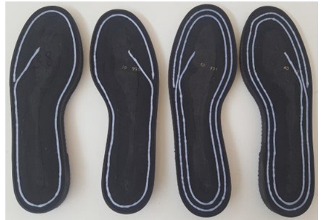
FIGURE 11. Adhesive toolpath, single (left) and double (right) parallel.
