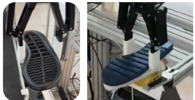
FIGURE 16. Left: grasping the outsole from the conveyor. Right: grasping the outsole to do the assembly.
