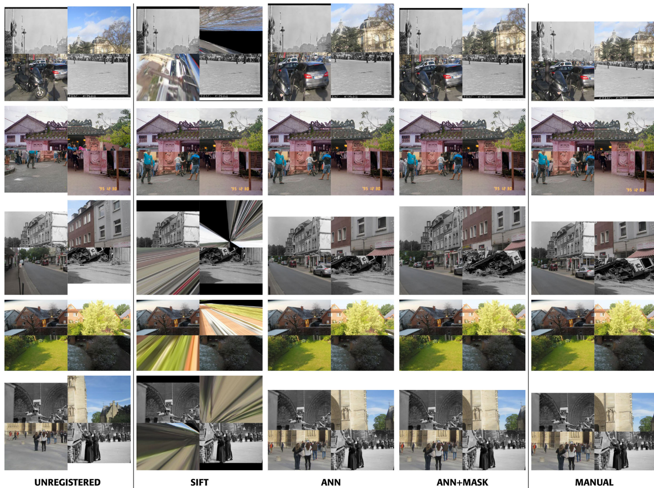
FIGURE 7. Registration results of the images and feature points shown in Figure 6. Registration results of the ANN and ANN+MASK method are comparable to the ground truth MANUAL method. SIFT fails in several cases resulting in worse images than UNREGISTERED. ANN and ANN+MASK differ, since ANN+MASK registers the AOI better but may register other areas worse compared to ANN. See Figure 6 for license information.
