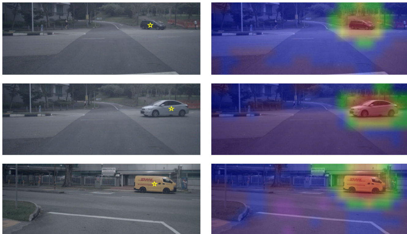
FIGURE 3. Cosine similarity of the features on the image feature map. We input the images into the CNN backbone ResNet-18 [28] and derive latent feature maps with a 256-channel vector on each pixel. Then we choose one vector located on the vehicle (the yellow star) as the query and calculate the cosine similarity between the query and others. The temperature of the heatmaps visualizes the similarity values.
