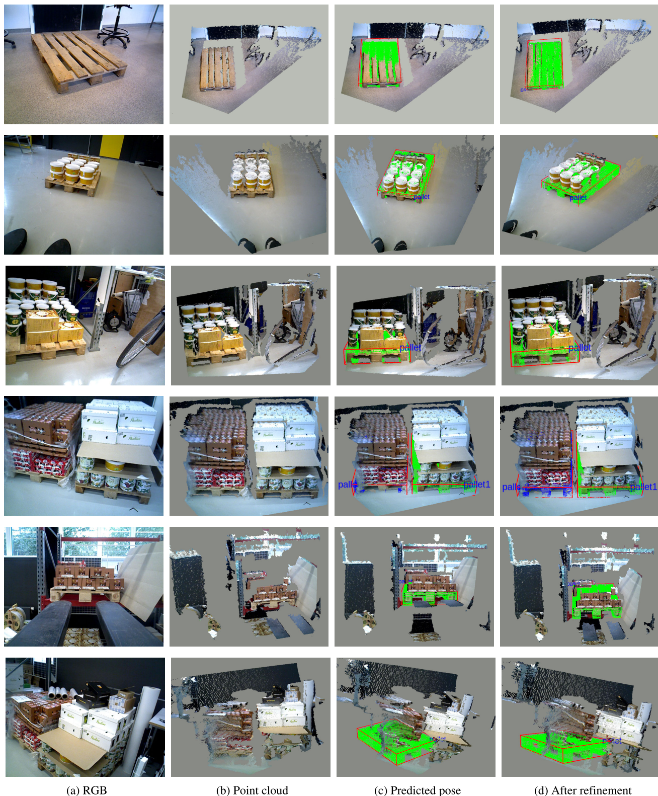
FIGURE 6. Qualitative results of the proposed method. The first two columns show color images and point clouds. The third column presents the visualization of the predicted pallet pose using 3D bounding boxes, with green points representing the 3D pallet model points aligned to the scene based on the predicted pose. The fourth column showcases the visualization of the refined predicted pose using the Iterative Closest Point (ICP) algorithm [30].
