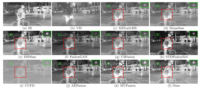
FIGURE 7. Qualitative comparison of the AMFusionNet with seven state-of-the-art methods on FLIR_09488 . For a clear comparison, we selected a salient region (i.e., the red box and green color box) in each image and zoomed in on it using the same color box, respectively. From top to bottom (from left to right): infrared and infrared image pair, fusion results of the CUFD [53], MDLatLRR [13], Densefuse [51], DIDfuse [63], FusionGAN [30], U2Fusion [34], STDFusionNet [78], AEFusion [64], MUFusion [65], and AMFusionNet.
