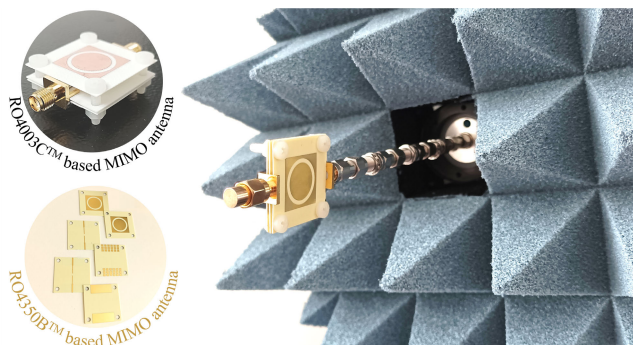
FIGURE 10. Fabricated MIMO antennas.
