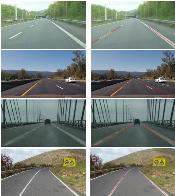
FIGURE 6. The result images of hough transform and lane extraction.
