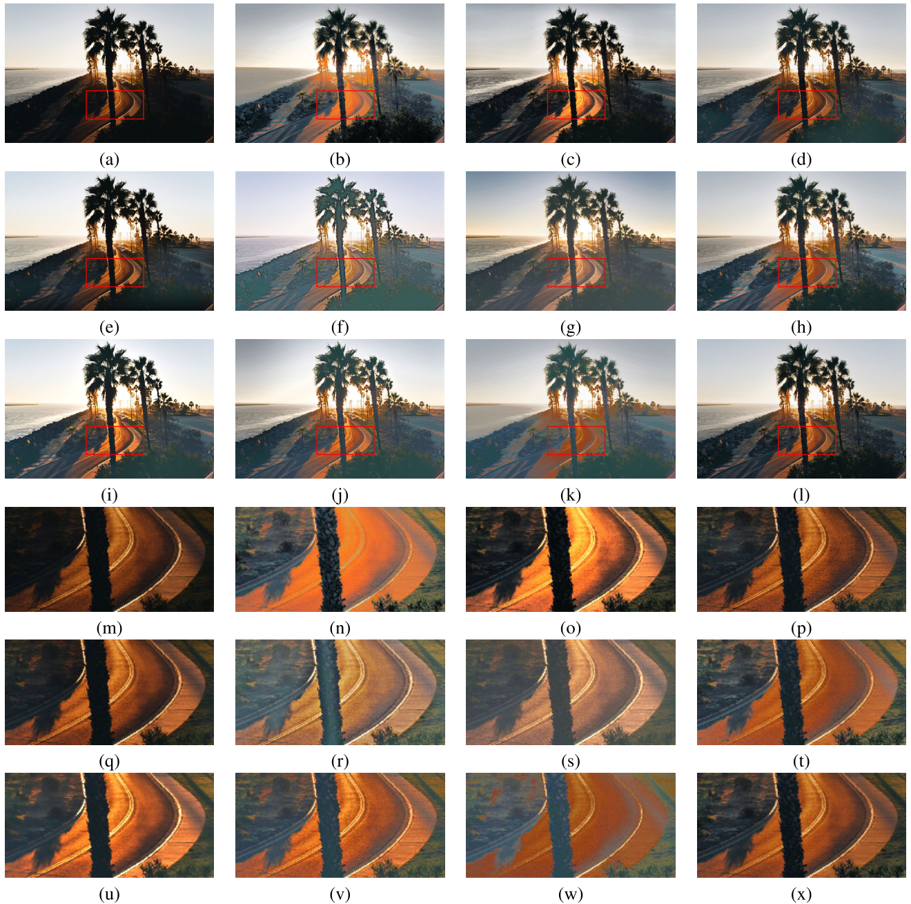
FIGURE 6. Experimental results for image 2. (a) is the input image. (b)–(l) are the results of HE, CLAHE, Wang et al.’s method, SRIE, ZERO-DCE, Ueda et al.’s method, Akai et al.’s method, Hao et al.’s method, Buades et al.’s method, Mukaida et al.’s method and the proposed method, respectively. (m)–(x) are the enlarged excerpts of boxed regions of (a)–(l).
