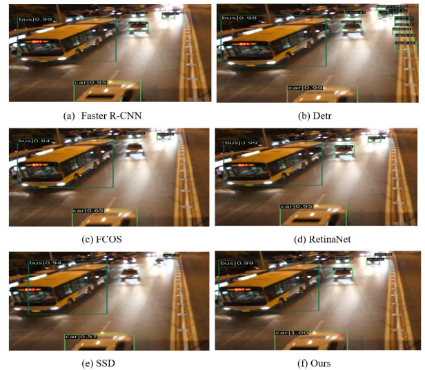
FIGURE 7. Detection results of the headlight scene from UA-DETRAC. (a) Faster R-CNN, (b) Detr, (c) FCOS, (d) RetinaNet, (e) SSD, (f) Ours.
