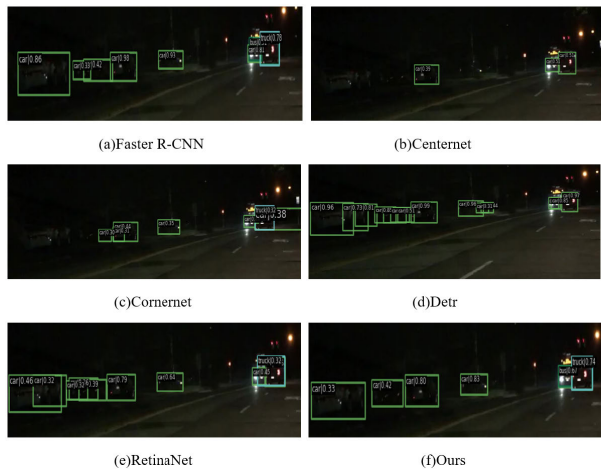
FIGURE 5. Detection results of dark scene from BDD100K. (a) Faster R-CNN, (b) CenterNet, (c) Cornernet, (d) Detr, (e) RetinaNet, (f) Ours.
