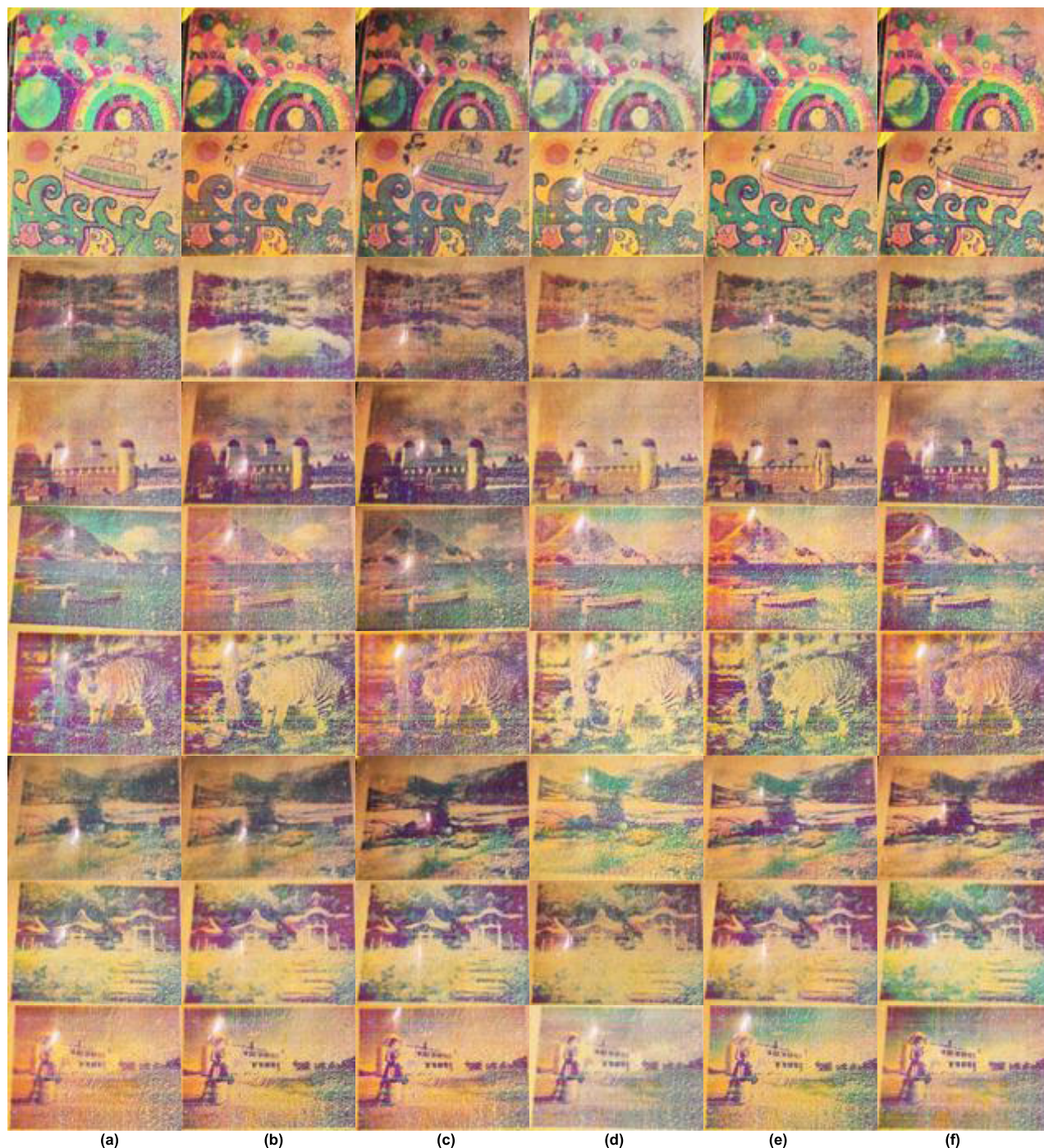
FIGURE 7. The display effect of CMY electrowetting electronic paper on images processed by different algorithms under the light source of 5000 K color temperature and 65500 Lux illumination. (a) RGB original images; (b) Du et al.; (c) Braik et al.; (d) Xu et al.; (e) Hu et al.; (f) Ours.
