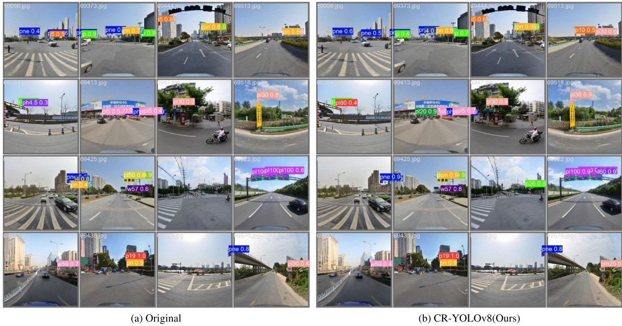
FIGURE 8. Visualization results of traffic sign detection on the TT100k dataset. (a) shows an example of detection on the benchmark network YOLOv8s. (b) is an example of detection on the CR-YOLOv8.
