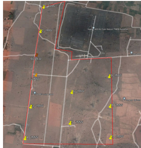
(b) Layout of repowered wind farm with nine 1 MW turbines
