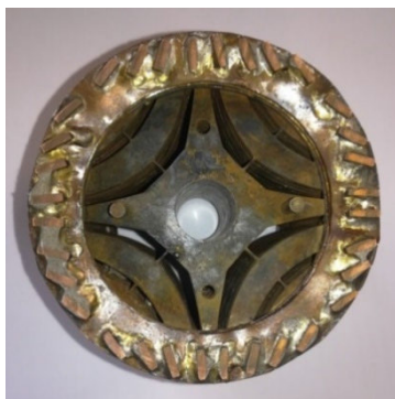
FIGURE 18. Cross section view of the soldered the squirrel cage bars.
