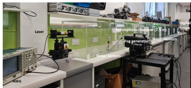
FIGURE 4. Representative photograph of the atmospheric chamber under use in this test. Alternate equipment was used in this paper as described in the text.
