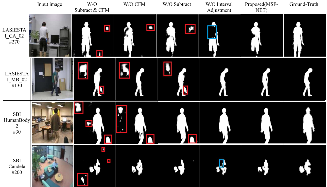
FIGURE 8. Ablation study qualitative evaluation result (red box: when the background is incorrectly classified as foreground, blue box: when the foreground is incorrectly classified as background).
