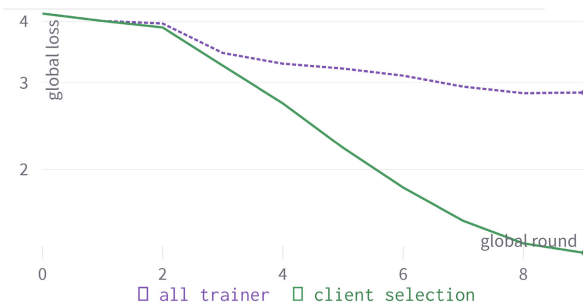
FIGURE 15. BCFL's global model loss graph where client selection was performed by giving additional scores to DID-certified trainers (solid) and BCFL's global model loss graph with no client selection (dashed).
