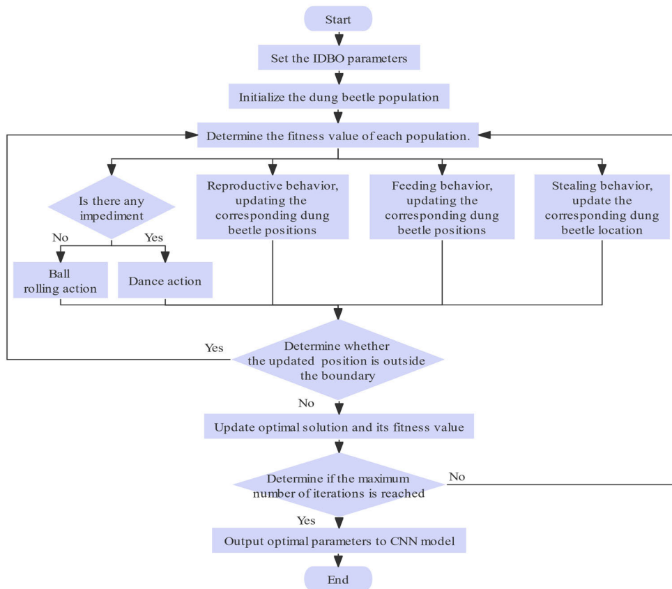
FIGURE 4. Optimization process of CNN parameters using IDBO algorithm.
