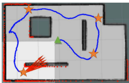
FIGURE 5. Simulation environment for the comparison of different path planning algorithms, with the starting point fixed at the center of the map (green triangle) and four fixed goals shown as orange stars.
