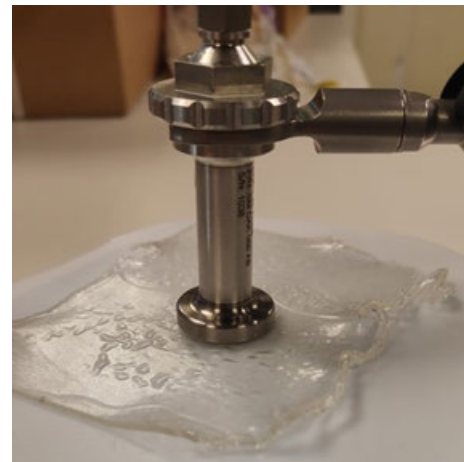
FIGURE 3. Coaxial probe for measuring dielectric properties of the custom-synthesized materials.
