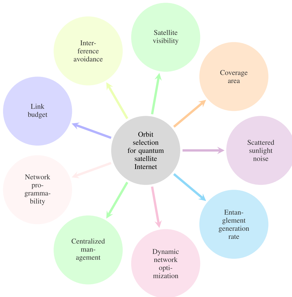
FIGURE 3. Design parameters for orbit selection in quantum satellite networking.
