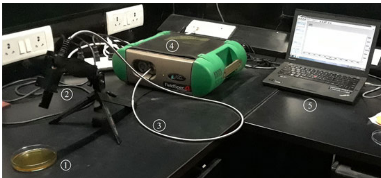
FIGURE 2. The experimental setup used in this study to acquire the reflectance Vis-NIR spectra of the honey and sugar samples. (1) Honey sample, (2) Sensor lens, (3) Optic fiber probe, (4) ASD Spectroradiometer, (5) Laptop.
