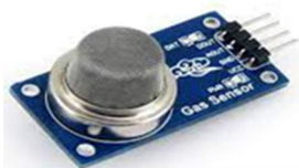
FIGURE 2. Chemical sensor on chip.
