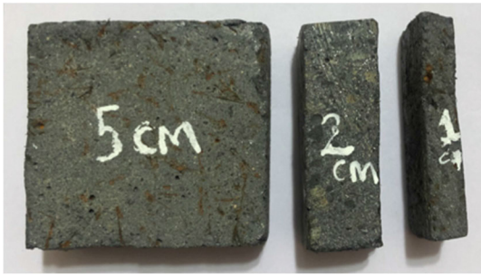
FIGURE 1. Conductive concrete with thicknesses of 5cm, 2cm and 1cm respectively.
