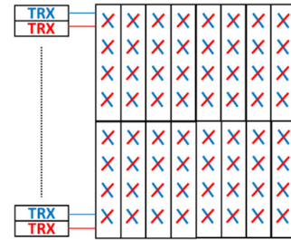
FIGURE 6. Antenna array with 8 \times 8 cross-polarized antenna elements formed in 16 sub-arrays. Each sub-array is connected to 2 TRX (1 TRX per polarization).
