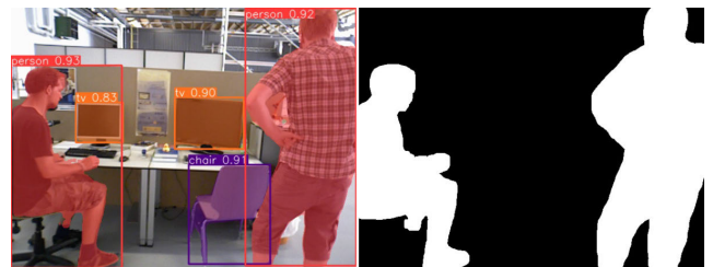
FIGURE 2. Target detection and instance segmentation based on YOLOv8.
