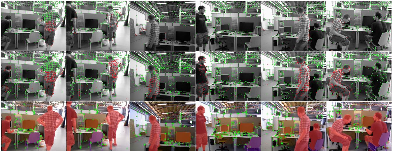
FIGURE 5. Displays the tracking comparison results of different algorithms. From left to right are the results of frames 44, 68, 216, 499, 663 and 759. The top row presents the tracking results obtained using the traditional motion consistency check algorithm. The middle row showcases the performance of the improved motion consistency check algorithm proposed in this paper. The bottom row represents the comprehensive tracking results achieved by combining this improved algorithm with the YOV0v8 semantic segmentation network.
