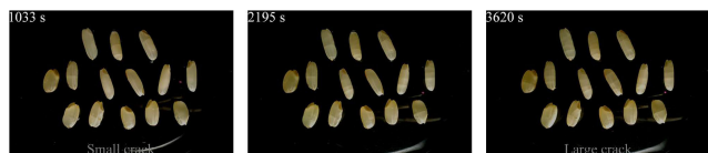
FIGURE 1. The crack formation process within brown rice kernels.
