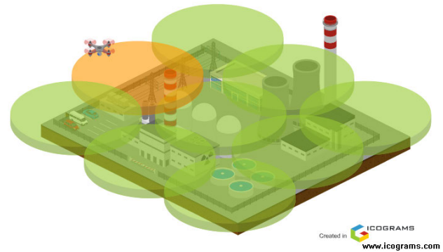
FIGURE 1. Concept of a distributed detection system based on an example allocation of nine sensors for the protection of an industrial facility. The arrangement of the sensors can be selected so that the detection areas overlap. Intrusion detection allows coarse localisation to take place immediately.
