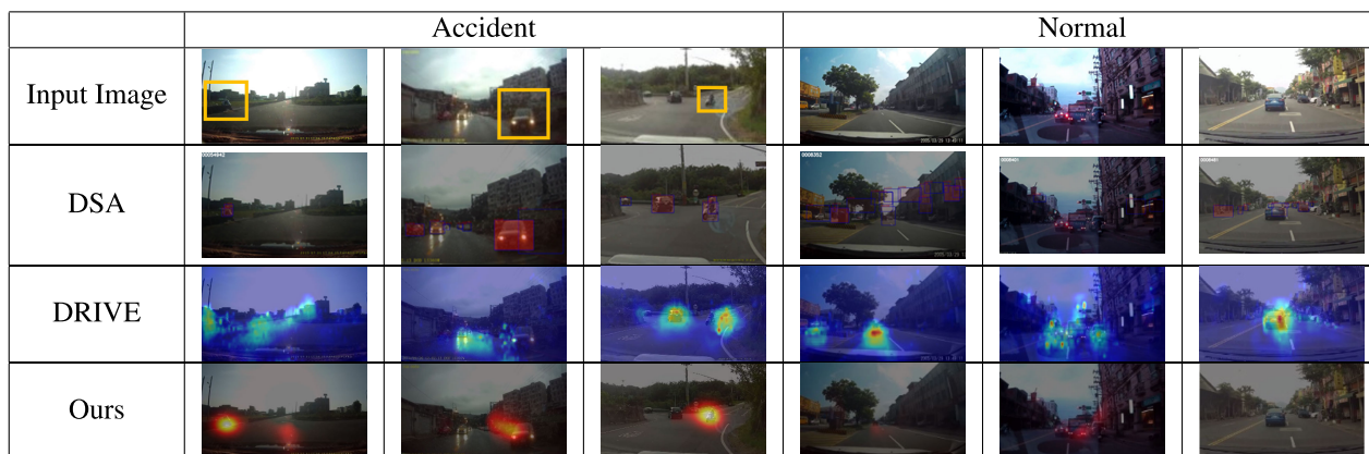
FIGURE 6. Visual description of the model in DAD. Risk factors for the input image are shown in yellow. The three on the left are accident scenes, and the three on the right are normal scenes. In the proposed method, only the areas determined to be risk factors are visualized using a heat map.
