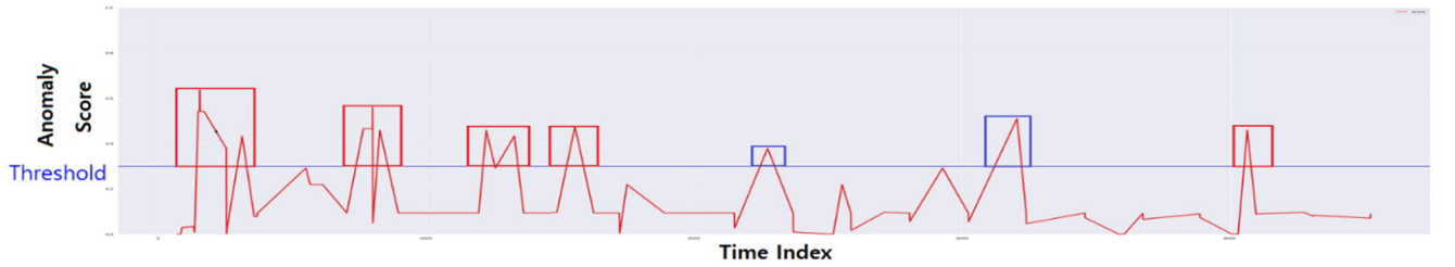
FIGURE 16. Anomaly score plot including attacks #1 to #10 in the SWaT dataset. After arranging the calculated train data anomaly scores in descending order, the “Threshold” indicated by the blue line was set to the top 10%. Of the ten attacks, red boxes indicated detected eight attacks, and blue boxes indicated two false alarms.
