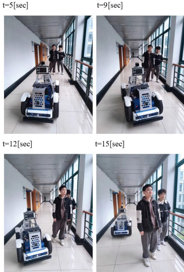
FIGURE 20. Actual photograph of the dynamic obstacle avoidance test in a narrow corridor.
