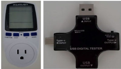
FIGURE 8. Energy tester equipment (Left is a tester for non-USB powered devices and Right is a tester for USB powered devices).
