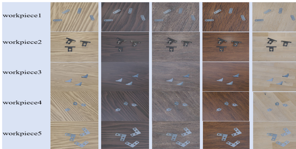
FIGURE 11. Virtual images of the workpiece created at different positions and with different backgrounds by the virtual engine.
