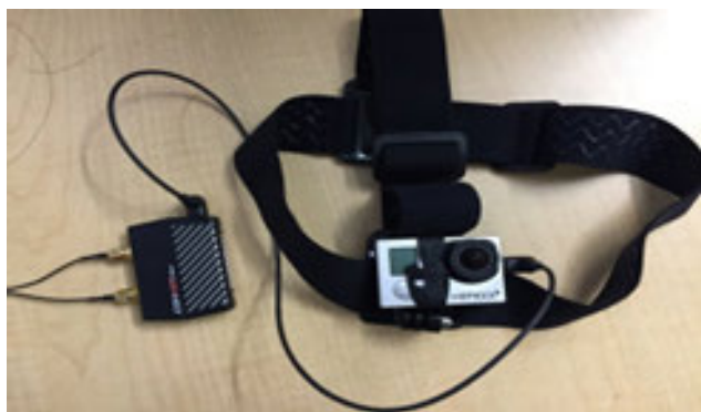
FIGURE 5. Camera device and image streaming device.
