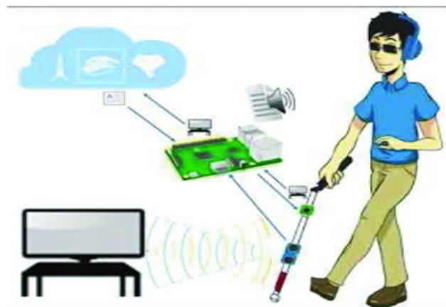
FIGURE 6. Smart e-stick using android application and cloud vision API.
