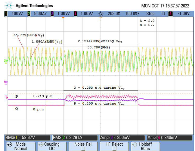
FIGURE 17. Experimental result illustrating P and Q injection with CACC mode ( k = 2.0 , and m = 0.7 ).
