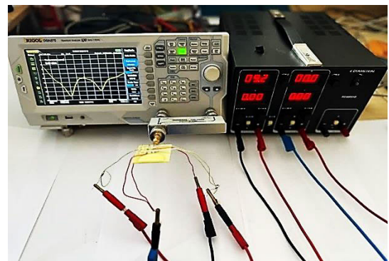
FIGURE 13. Reflection coefficient measurement equipment setup.
