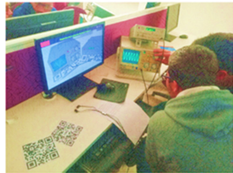
FIGURE 6. Students can interact with the virtual oscilloscope and function generator on the screen using the computer mouse. The mouse left click to press the buttons and the scroll to rotate the knobs. Source: Adapted from [58].
