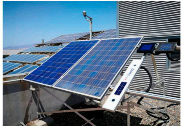
FIGURE 4. Shows a testing facility for outdoor PV panels with clean and dirty panels [52].
