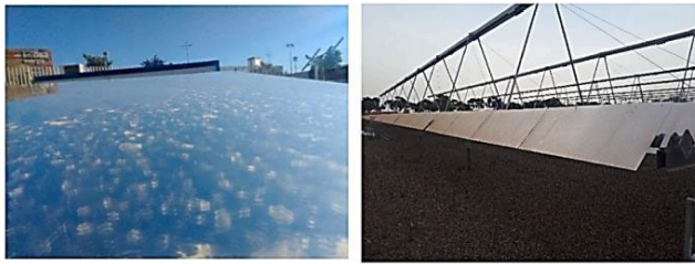
FIGURE 14. Shows the Very-High Concentration Solar Tower at IMDEA Energy in Spain, where the heliostat is affected by a light rain(Left); and the Fresnel mirrors at the Green Energy Park in Morocco, which have experienced a red rain event (Right) [77].
