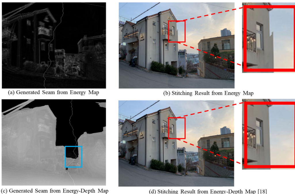
FIGURE 12. Comparison of image stitching results using the energy and energy-depth maps: (a) seam generated from energy map (b) stitching result from energy map (c) seam generated from energy-depth map (d) stitching result from energy-depth map.
