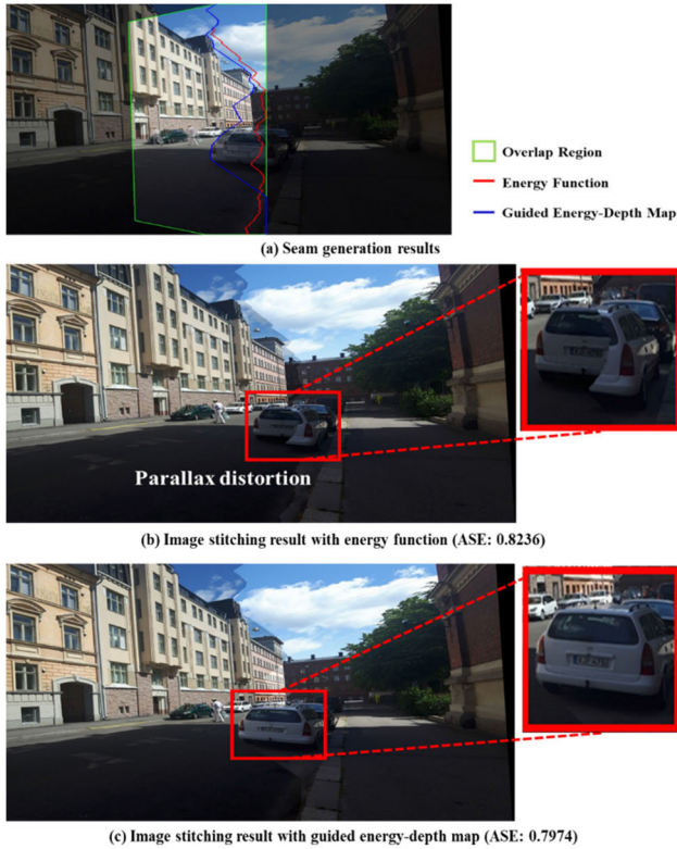
FIGURE 24. Seam generation and image stitching results of energy function and GED map for greater parallax distortion: (a) seam generation results (b) image stitching result with energy function, ASE: 0.8236 (c) image stitching result with GED map, ASE: 0.7974.
