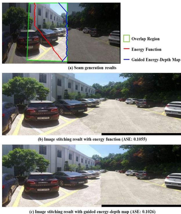
FIGURE 22. Seam generation and image stitching results of energy function and GED map with little parallax distortion: (a) seam generation results (b) image stitching result with energy function, ASE: 0.1055 (c) image stitching result with GED map, ASE: 0.1026.
