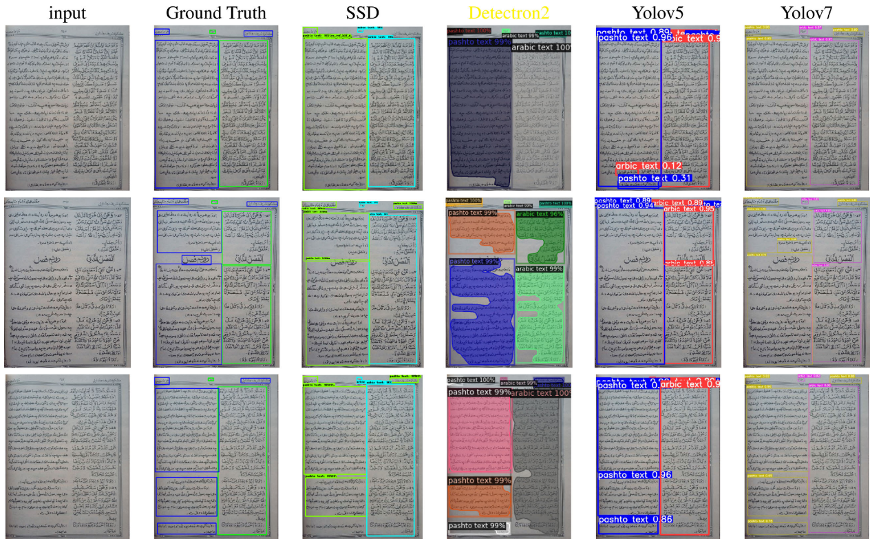
FIGURE 7. Visual results for SSD, Yolov5 and Yolov7 compared to the original input image along with ground truth.
