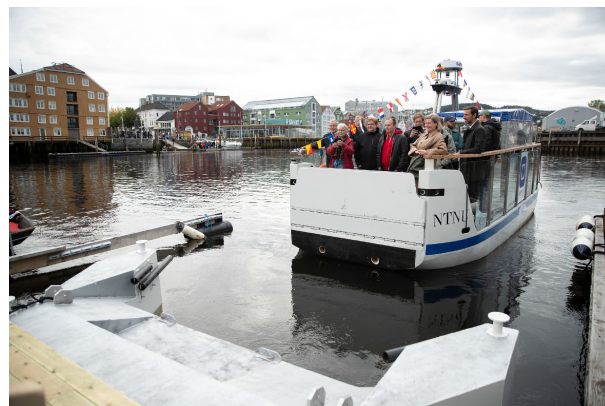
FIGURE 1. The autonomous urban passenger ferry milliAmpere2 performing automated docking in the Canal in Trondheim, Norway on September 22, 2022. Photo: Kai T. Dragland / NTNU.
