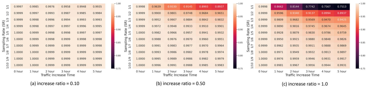
FIGURE 7. Correlation values when the sampling rate (SR) is changed at the traffic increase event. Darker colored areas on the heat map indicate a significant decrease in correlation values. The correlation value was computed using (5).
