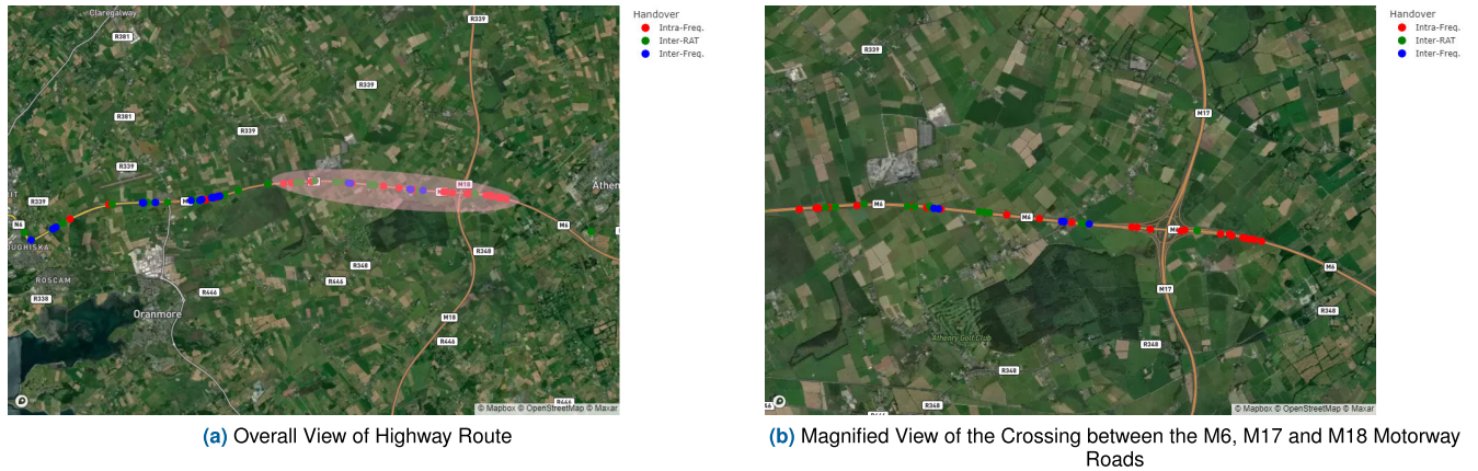
FIGURE 12. Handover type maps of highway driving route to and from Athenry town for the 5G NR-enabled GW1400 Device (centred at 53.299666, -8.903497) (Map data ©2023 mapbox).
