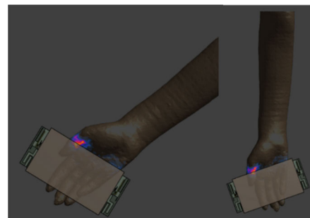
FIGURE 24. Smartphone MIMO antenna system placed on a human hand model.
