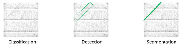
FIGURE 4. Photovoltaic micro-crack detection via computer vision.
