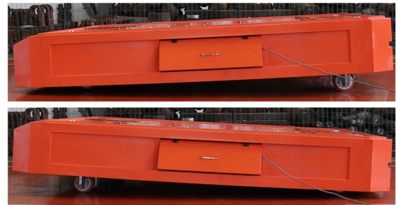
FIGURE 11. Demonstration of the rotational DOF around the Y-axis.
