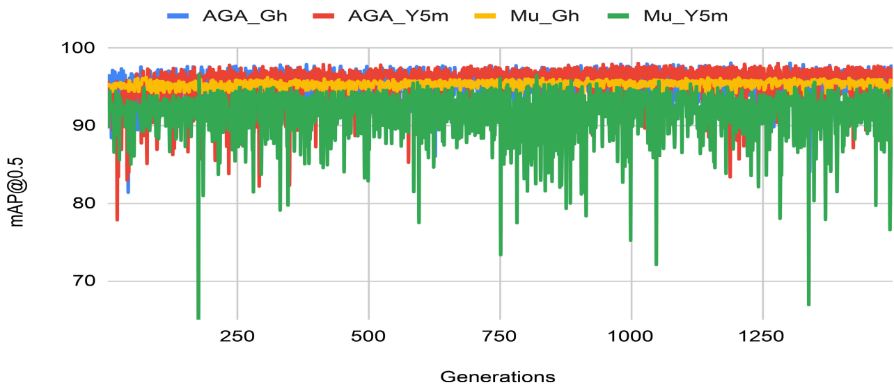
FIGURE 10. The results obtained from conducting tests involving the application of the adaptive genetic algorithm and YOLOv5 based mutation technique over a period of 1500 iterations on our dataset. AGA_Gh- Adaptive Genetic Algorithm using Ghost network and FPN, AGA_Y5m- Adaptive Genetic Algorithm using YOLOv5m, Mu_Gh - Mutation based evolution using Ghost network and FPN, Mu_Y5m- Mutation based evolution using YOLOv5m.
