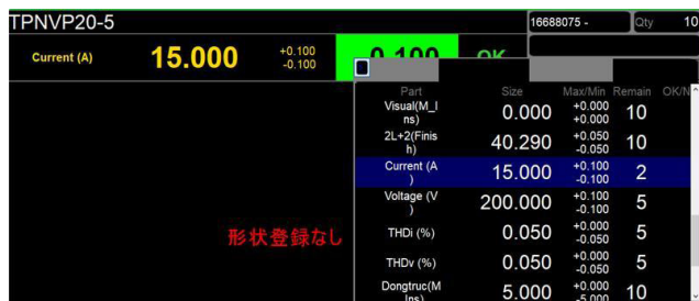
FIGURE 23. Power quality parameter online inspection screen.
